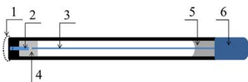
Fig. 1. Scheme of the platinum disc electrodes. 1—bioselective membrane, 2—platinum wire, 3—internal conductor, 4—Wood alloy, 5—epoxy resin, 6—contact pad.
